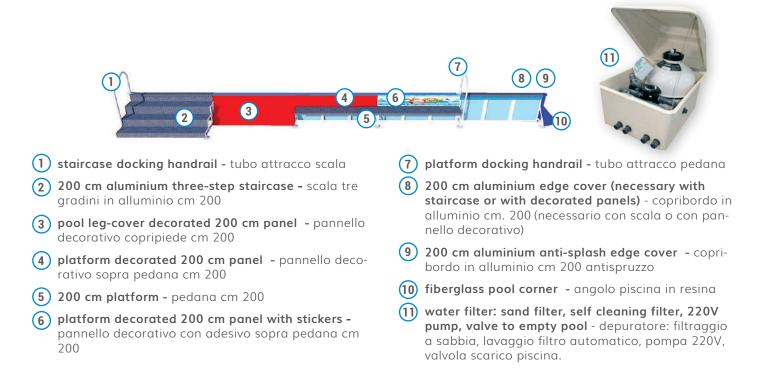
Bumper boat pool is built with modular units and it can be easily adapted to your space needs. Basic versions can be equipped with many accessories as shown on the next page. Decorations and scenery will make it a special attraction!
